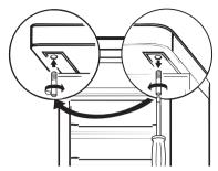
Carefully slide the door onto the top bearing pivot and close.
